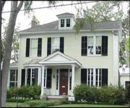
The window shutters of these two houses are original and properly fit the windows. The house on the left illustrates original shutters that are properly sized and hung for paired windows and a bay window.
