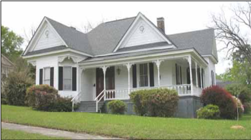
The house at the corner of Fifth Street and Missouri Avenue has both hip and gable roofs which is very typical of the Queen Anne style.
